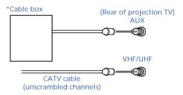
For this set up, you can switch between scrambled channels (through your cable box), and normal (CATV) channels by pressing TV ANT on your remote control. Notes:
